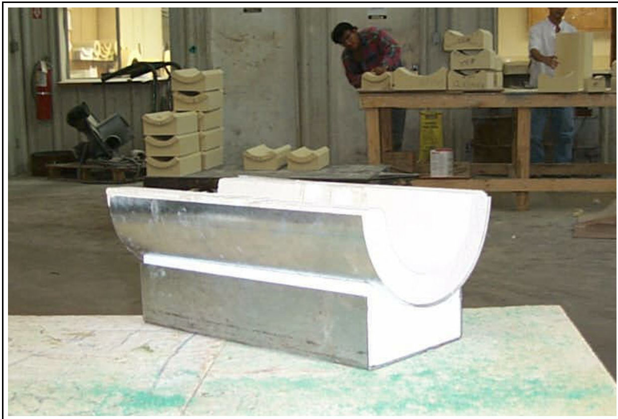
sting Shoe made of Calcium Silicate for hot service
