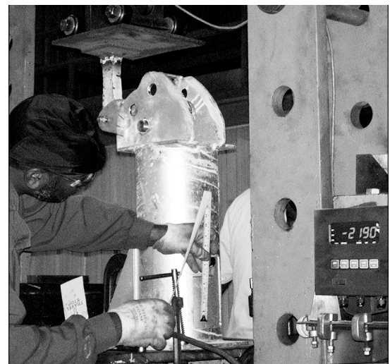
PTP 100-F TYPE CONSTANT UNDERGOING LOAD TESTING
