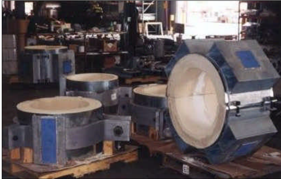
Hot Insulated Supports with Teflon Slide Plates
