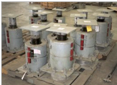
Variable Spring Supports Ready For Shipment
