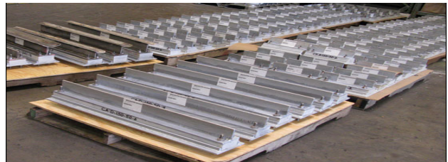
Cryogenic Pipe Supports with Micarta® Insulation for an LNG Plant
