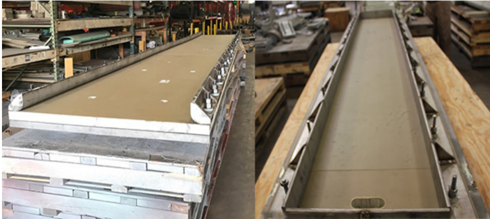
Micarta® Block Assemblies for Placement Beneath a Saddle Support of a Vessel
