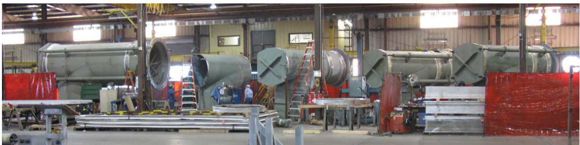
Pressure Balanced Metallic Expansion Joints During Fabrication in the U.S. Bellows Shop
