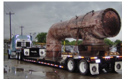
A Refurbished 54" Pressure Balanced Elbow Turbine Crossover Expansion Joint Being Shipped
