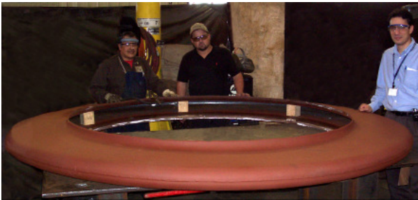
78" Diameter Thick-Wall Flanged and Flued Head Expansion Joint
