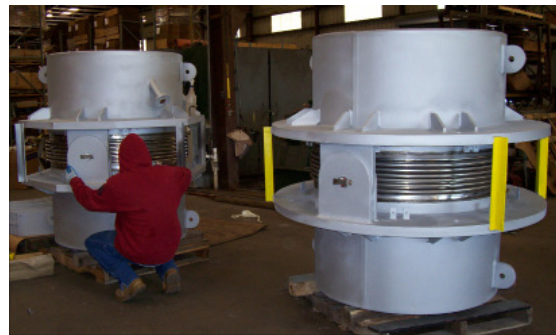
43" Hinged Expansion Joints with 5" Thick Refractory Lining
