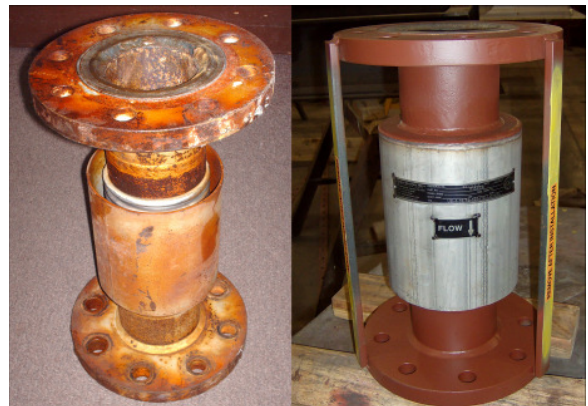
Refurbished Single 4" Diameter Expansion Joint in One Day
