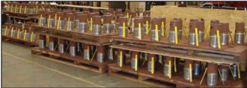
6" Single Expansion Joints for Installation in a Heater for a Delayed Coker Unit
